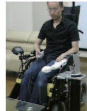
Autonomous running chair equipped with assistive service robotic arm
