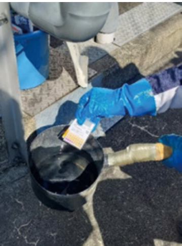
Water quality analysis during an environmental accident drill simulating a leakage accident at a laboratory wastewater treatment plant caused by an earthquake
