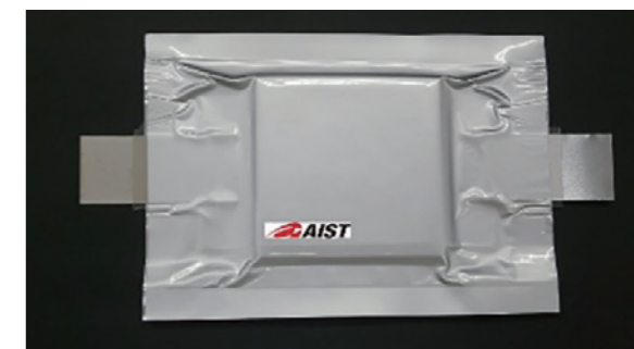
Prototype storage battery (8 Ah)
