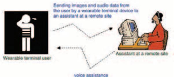
AIST is working on the development of a smaller, lighter, wireless wearable device and the application of the current communication infrastructure. The research efforts also focus on data expression methods that facilitate the improvement of information quality (image, sound etc.) from the assistant's point of view.
