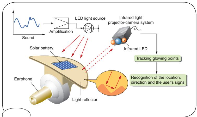
Mechanism of CoBIT: The device generates sound, receiving light signals which flash on and off in accordance with sound waveforms.
