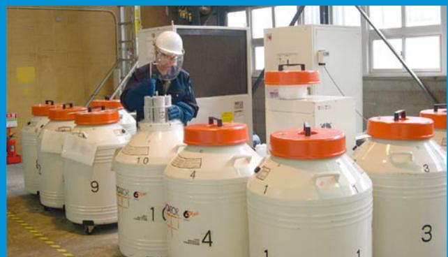
Containers for natural cores collected by the test boring from "the Off-Tokai ~ Off-Kumano"
