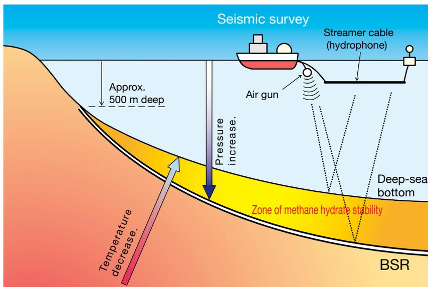
Figure 2 : Illustration of the reflection seismic survey
