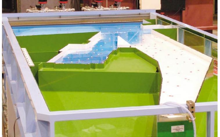
Photo : Hydraulic model experiment for destroying density stratification in Kitadomari Harbor, Osaka Bay
