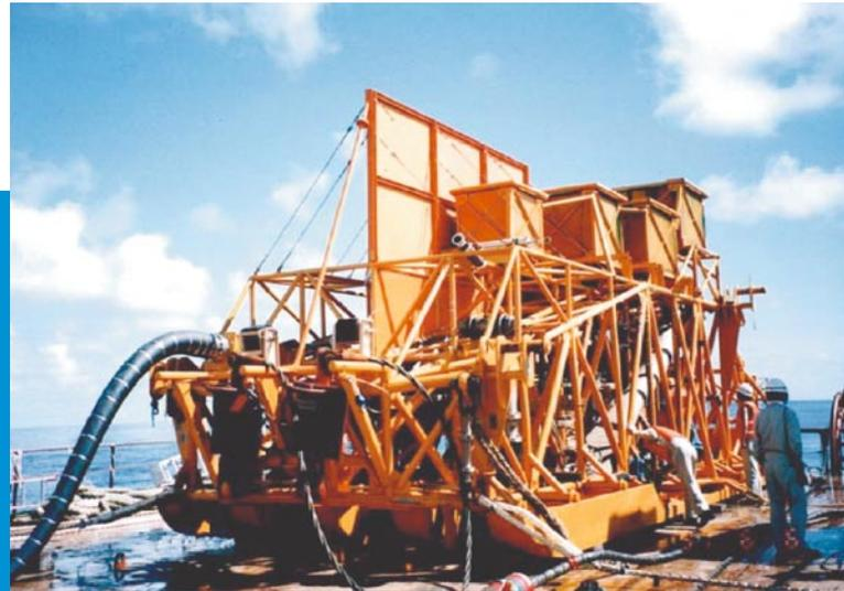
Photo : Nodule collector for ocean trial test, which was used by the large-scale project, "R&D of Manganese Nodule Mining System"
