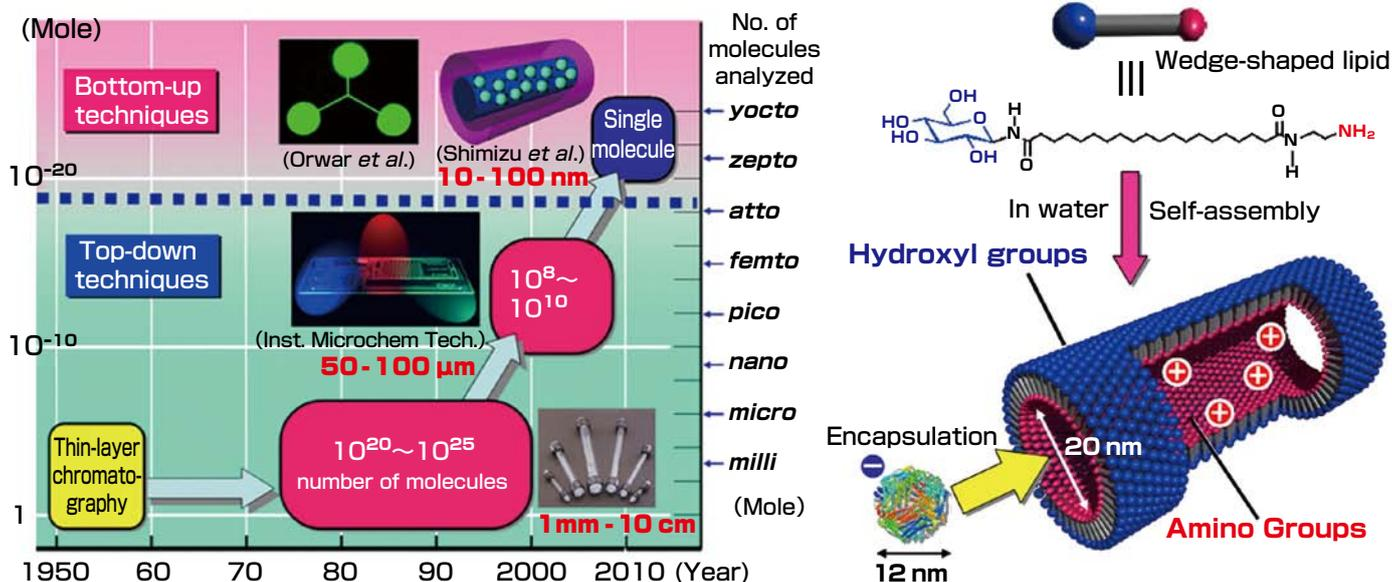
Figure. Chronological transition of miniaturization of hollow cylinder spaces, and the organic nanochannel consisting of molecules
