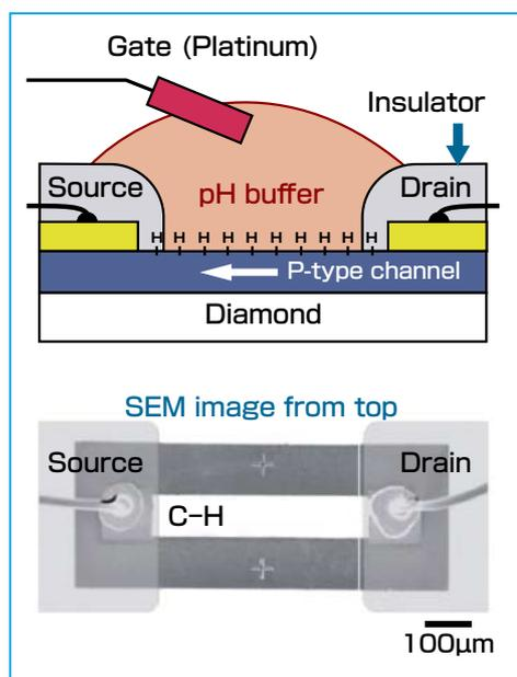
Figure 1. Schematic diagram of diamond pH sensor and SEM image
