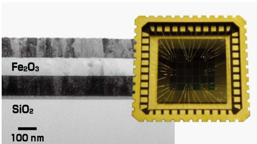
Figure 1. Cross sectional transmission electron microscope image of resistance random access memory structure consisting of iron oxide (left), and the prototype memory device of the same (right)
