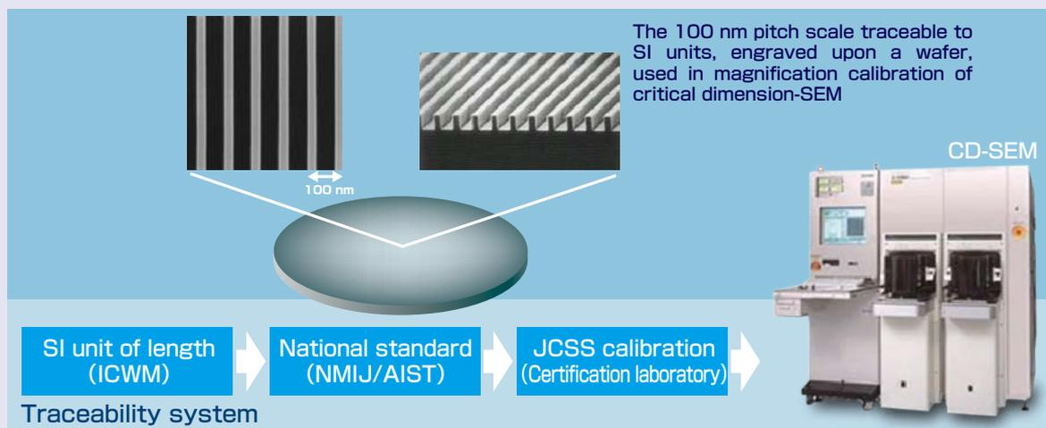
Figure. The 100 nm pitch nanoscale and the traceability system
