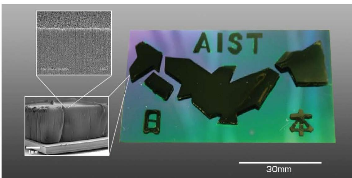
Photo 2. Carbon nanotubes which 'sustain Japan' (map of Japan made using vertically arranged SWNTs)
