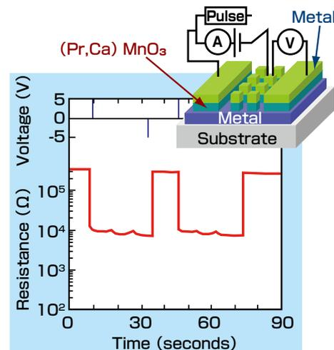
Figure 1. Colossal electro-resistance (CER) memory effect of perovskite manganese oxide
