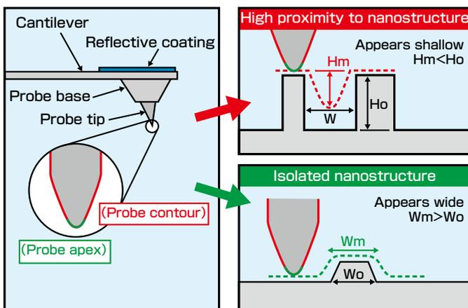
Figure. Schematic diagram indicating the problem in morphology measurement of nanosubstances (structures) using AFM
