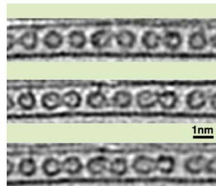
Figure 3. HRTEM image of ( $C_{60}$ - $C_3NH_7$ ) in SWNT, imaged continuously at 2-second intervals
