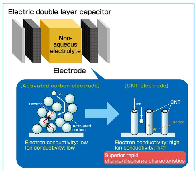
Figure 2. Comparison of activated electrode and CNT electrode
