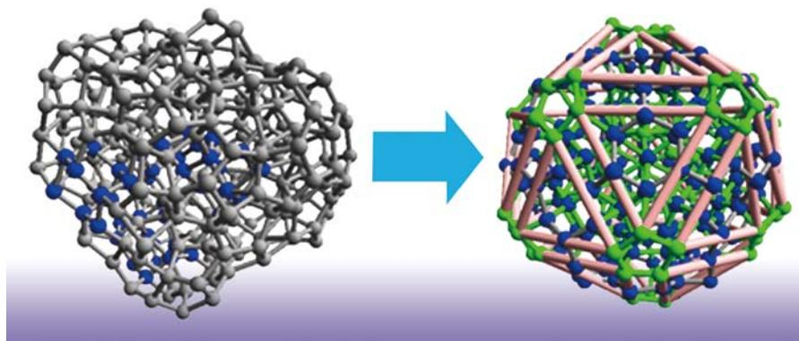
Figure 2. Simulation results of formation of a silicon regular icosahedral cluster
