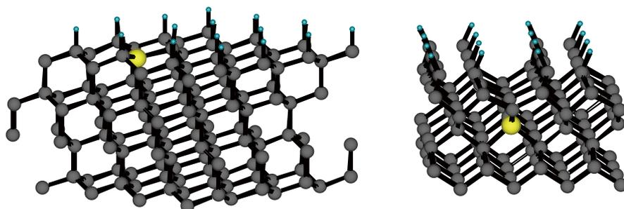
Figure 3. Optimized structure of phosphorous impurity atom (yellow) in surface region of hydrogenated diamond, Left: (111) surface, Right: (001) surface
