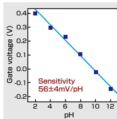
Figure 2. Sensitivity characteristics of diamond pH sensor
