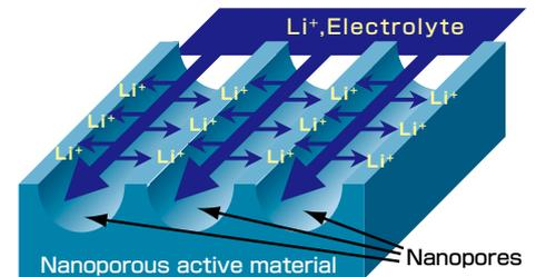
Figure 1. Image of diffusion path of lithium ions ( $\text{Li}^+$ ) through nanopores of a nanoporous active material
