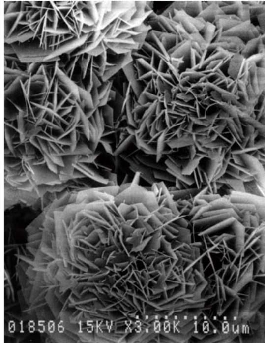
Photo. Electron microscope image of calcification by a phosphophoryn applied on agarose beads (Robust growth of apatite crystal was observed)
