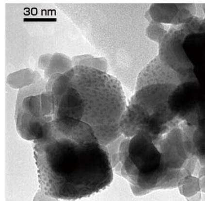
Photo. Palladium-supporting titanium oxide prepared by photodeposition
