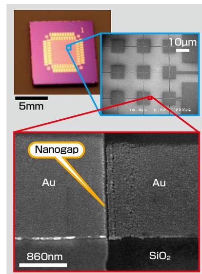
Figure 1. A chip integrated with 800 nanogap electrodes and its SEM photograph magnifying a nanogap part (molecule-sized gaps are constructed)
