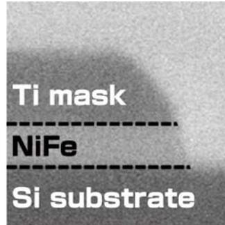
Figure 2. Cross sectional scanning electron microscope image of structure of NiFe (Permalloy) processed by reactive ion etching using Ti (titanium) masking (black dotted line has been added to show boundaries between materials)
