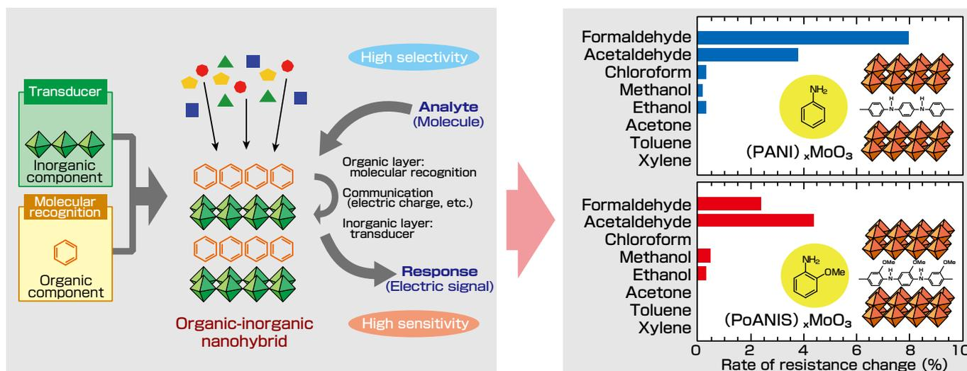
Figure. The concept of the organic-inorganic nano hybrid sensor, and response sensitivity to VOC of the organic/molybdenum oxide thin film element prepared
