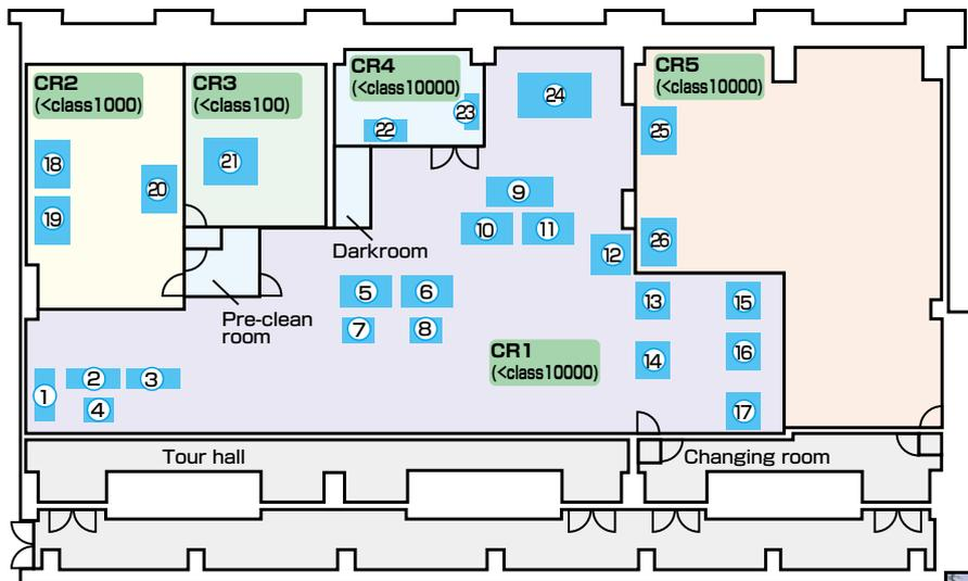
Equipment layout in clean room (CR) and exterior of AIST Nano-Processing Facility (AIST-NPF)
