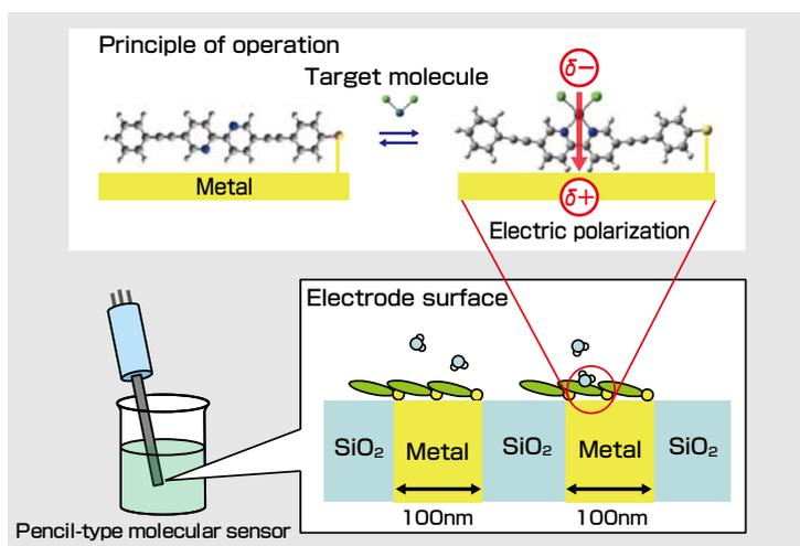
Figure 2. Electrode modification and principle of operation of pencil-type molecular sensor used in solution (when the target molecule was captured by the organic molecule adsorbed on the nanoelectrode surface, electric polarization is induced on the surface, and this change is detected)
