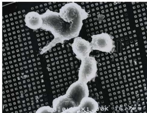
Figure 1. Method for preparation of nanopillar sheet using nanoimprinting technology (left) and electron microscope photograph of HeLa cells cultured upon nanopillars (diameter 0.5  $\mu\text{m}$ ) (right)
