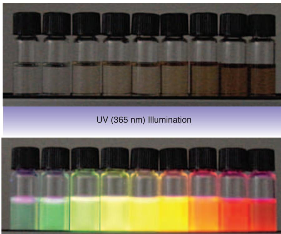
Fig. 2 Fluorescence from CdSe nanoparticles with various diameters that are synthesized by heating during 2-140 s at 300°C. Smaller particles (ca. 2 nm) prepared with shorter heating-time emit blue-green light, whereas larger ones with longer heating time emit red light.
