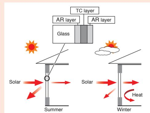
Schematic structure and performance of the window.
