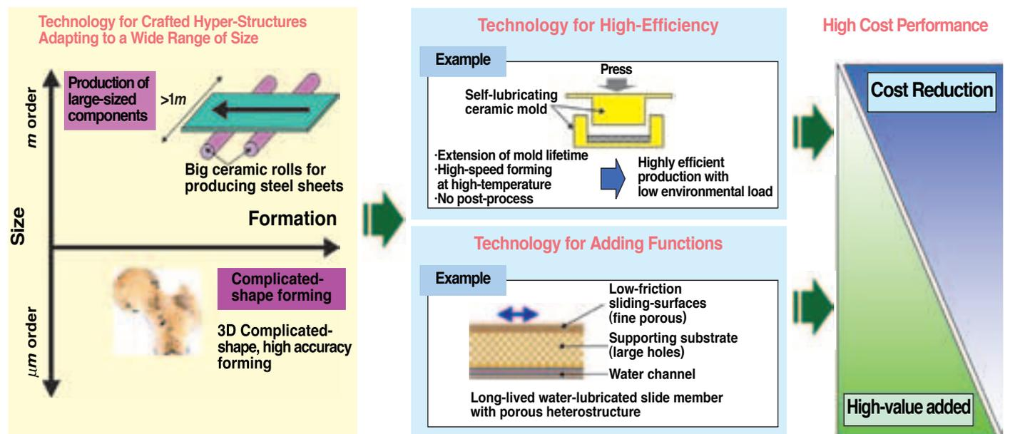
Fig. 3 Development of tailored manufacturing process.
