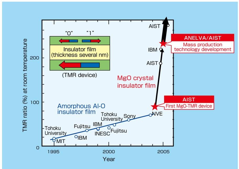
History of the performance improvements of tunnel magnetoresistance (TMR) devices which convert magnetic data to electric data
