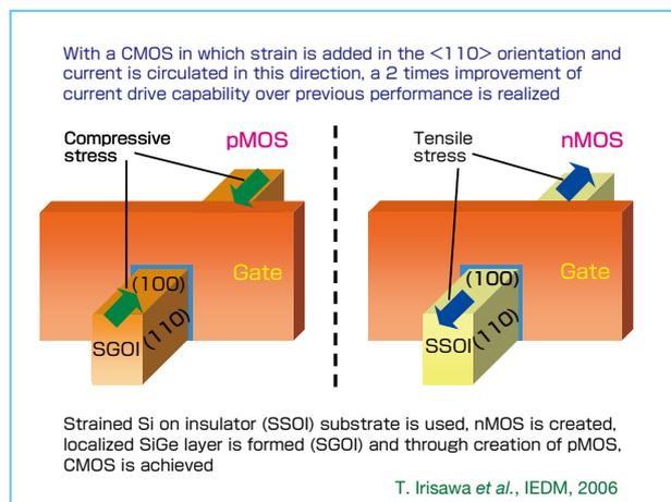
Figure 7: Most effective structure for uniaxial strained multigate CMOS (modulation of sub-band structure)
