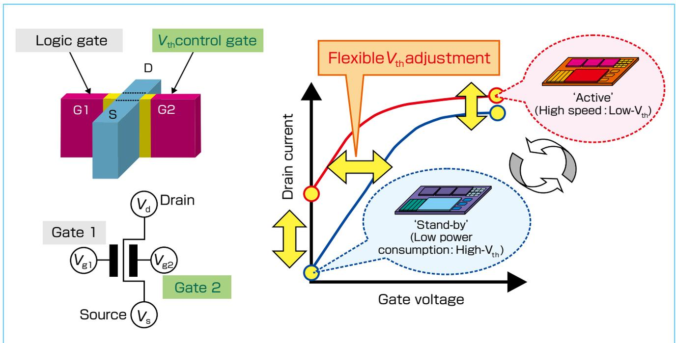
Figure 3: Unique function of the 4-terminal double-gate MOSFET (4T-XMOSFET) By flexibly controlling  $V_{th}$ , both high speed during the active state and low power consumption during the standby state are achieved.
