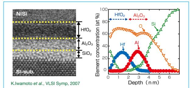
Figure 9 : Cross-sectional transmission electron microscope photograph of high-k gate insulator film consisting of a gate stack comprised of 2 layers: HfO<sub>2</sub>/Al<sub>2</sub>O<sub>3</sub> (left), and profile of composition of HfO<sub>2</sub>/Al<sub>2</sub>O<sub>3</sub>/SiO<sub>2</sub> layers by depth
