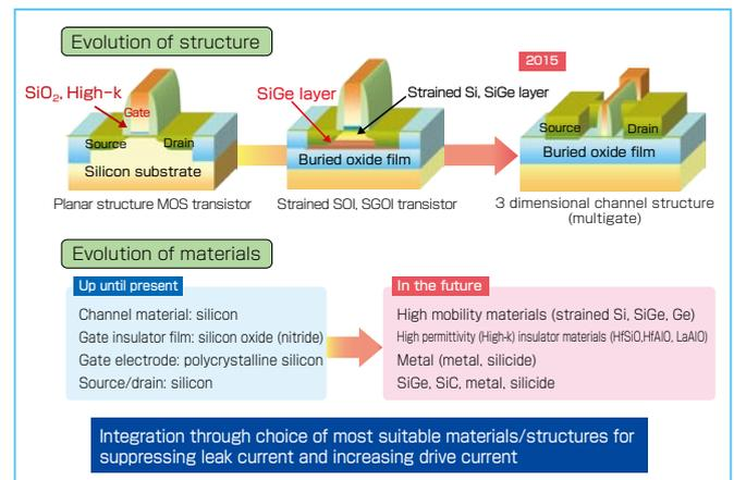
Figure 4 : New materials and structures aimed at improving transistor performance
