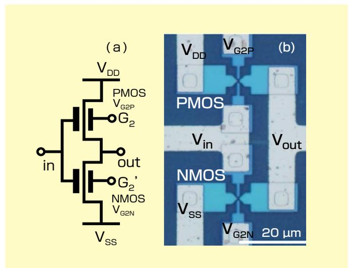
Figure 2 : CMOS inverter that uses 4-terminal double-gate MOSFETs (4T-XMOSFETs)
