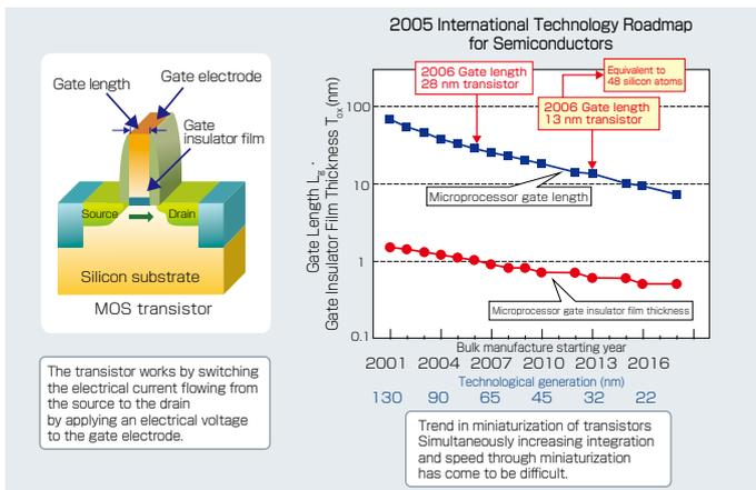
Figure 3 : Miniaturization towards a 10 nanometer gate length MOS transistor
