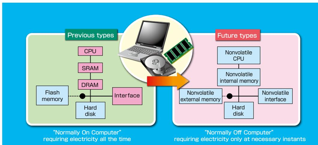
If nonvolatile devices, which do not lose their data even if the power is turned off, can be developed, then a great reduction in the electricity consumption of electronic data devices is expected.
