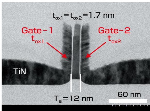
Figure 1 : Prototype 4-terminal double-gate MOSFET (4T-XMOSFET) Fabricated by using the anisotropic wet etching for the well standing-up fin channel, and the reactive ion etching (RIE) for the gate separation.
