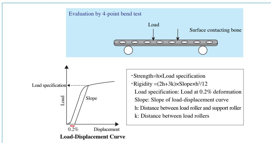
**Figure 1: Method for mechanical properties evaluation of bone plate**
