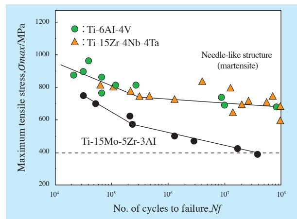
Figure 3: Comparison of fatigue characteristics of titanium alloys
