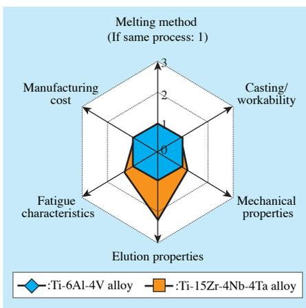
Figure 4: Comparison of titanium alloys
