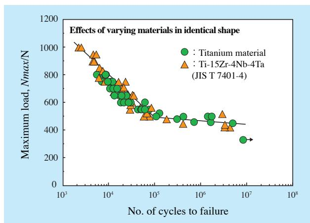
Figure 2: Results of 4-point bend test on straight plates
