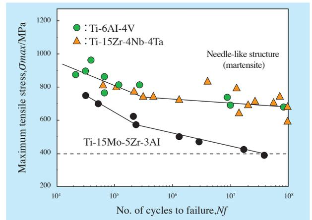
Figure 3: Comparison of fatigue characteristics of titanium alloys
