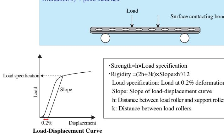
Figure 1: Method for mechanical properties evaluation of bone plate
