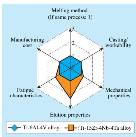
Figure 4: Comparison of titanium alloys
