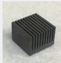
Solid phase-change-ceramics with metal dispersion for thermal storage
