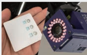
Simplified hemodiagnosis chip and measuring device of body functions
