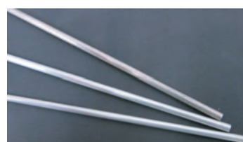
Long-fine Mg alloy tubes fabricated by developed tube extrusion method
