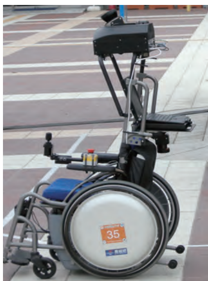
Fig.1 “Marcus” wheelchair with autonomous traveling capability Attached with sensors for creating 3D environmental maps on the upper rear of the chair
