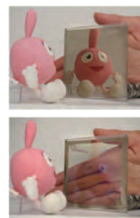
A newly developed switchable mirror coated with antireflection layer
