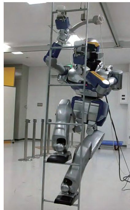
A humanoid robot climbing a fully vertical ladder using its two hands and two feet
