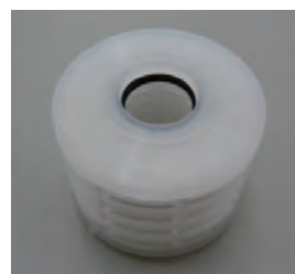
Nonwoven fabric cartridge filter impregnated with potassium zinc ferrocyanide
