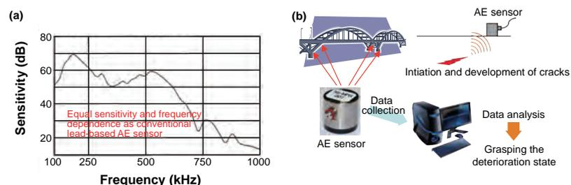
(a) Sensitivity of lead-free AE sensor to the frequency of mechanical vibration
