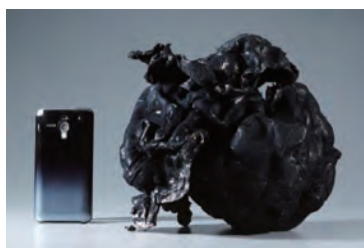
A lump of SWCNTs synthesized in the developed industrial production plant (compared to a smartphone)
