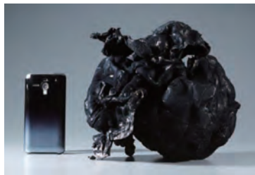
A lump of SWCNTs synthesized in the developed industrial production plant (compared to a smartphone)
