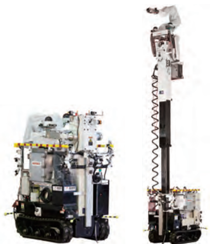
The high-access survey robot when driving (left) and when surveying (right)
