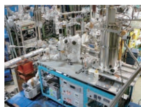
Fig.1 X-ray absorption fine structure spectrometer using 100-pixel superconducting tunnel junction array detector
