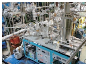
Fig.1 X-ray absorption fine structure spectrometer using 100-pixel superconducting tunnel junction array detector
