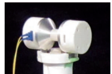
Proposed optical fiber link system and new bi-cone type antenna
