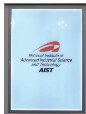
Fig. 2 A1-size (594×841 mm) transparent graphene sheet synthesized by microwave plasma CVD
