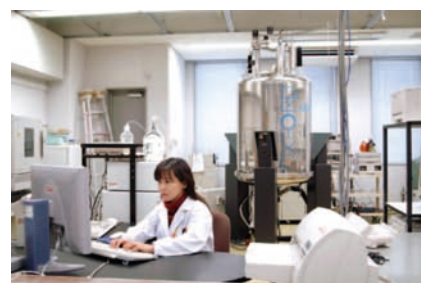
Nuclear magnetic resonance equipment (NMR) to analyze high-purity organic compounds
