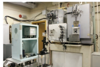
The national standard to calibrate the doseimeters for mammography radiation
