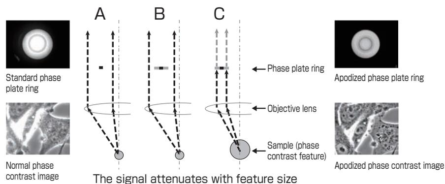
**Fig. 2. The principle of apodized phase contrast microscopy (left: phase contrast microscopy, right: apodized phase contrast microscopy)**
