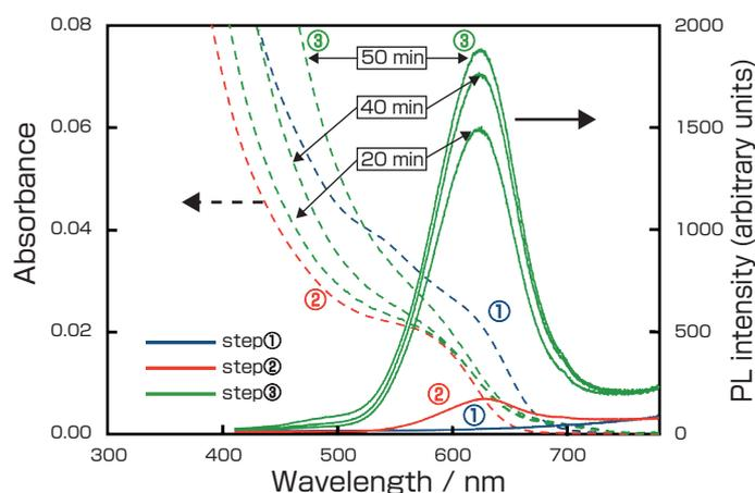
Changes in the absorbance (dotted lines) and PL spectra (solid lines) during the 3-step process of producing InP/ZnS NCs
