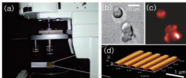
(a) Photo of a fluorescence microscope using the grating substrate
