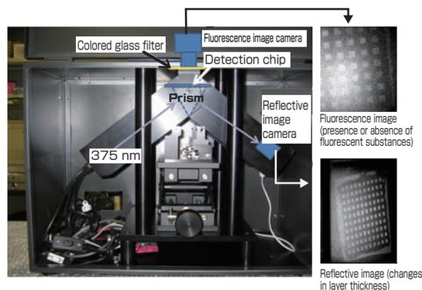
When light hits the detection chip at the waveguide mode oscillation angle, incident light intensity is enhanced at the surface of the optical waveguide (left schematic). The photos to the right show a prototype measurement system.
