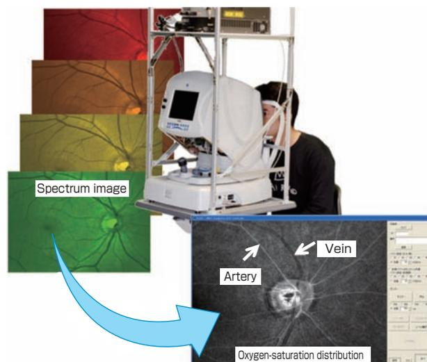
**Spectroscopic SLO apparatus we developed, captured spectral images, and the resulting image indicating the pattern of oxygen saturation levels in a normal fundus**
