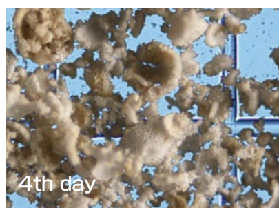
High pressure dissolution experiment of calcium carbonate settling particles (foraminiferal shell) The spheric shells are rapidly dissolved in sea water of high concentration of CO 2 .
