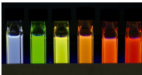
Figure 1: Fluorescence emitted from quantum dots. Blue fluorescence can be emitted from small particles of approximately 2 nm in diameter, green from ~3 nm particles, yellow from ~4 nm particles, and red from large particles of ~5 nm.
