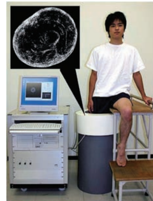
Figure 2: Cross-sectional imaging based on "Ubiquitous Echo".
