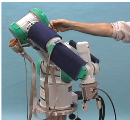
Photo 3: Contact-avoidance using the sense of touch
