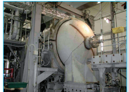
Photo. Sealed detonation chamber used to dispose of munitions.
