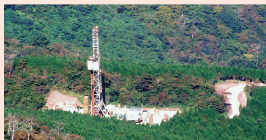
Photo Unzen Scientific Drilling site on the north-side slope of Unzen Fifty meter-high rig were set up in an area of approximately 2000 m 2 , and a road was constructed in the national forest. (Pictures provided by Professor Setsuya Nakada, Univ. Tokyo)
