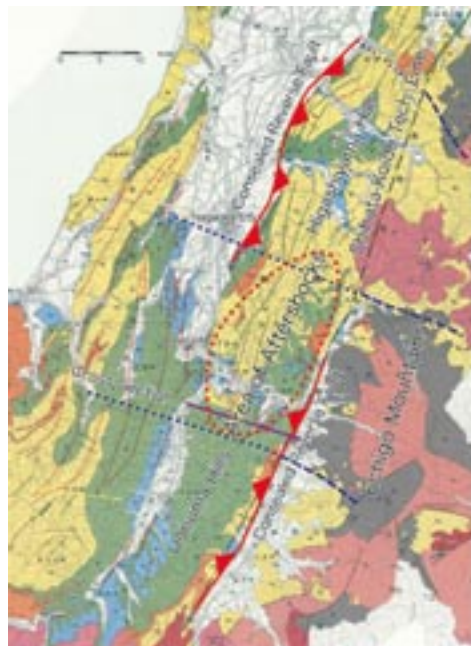
Geological structure and estimated cross section of the Mid Niigata Prefecture earthquake in 2004.
