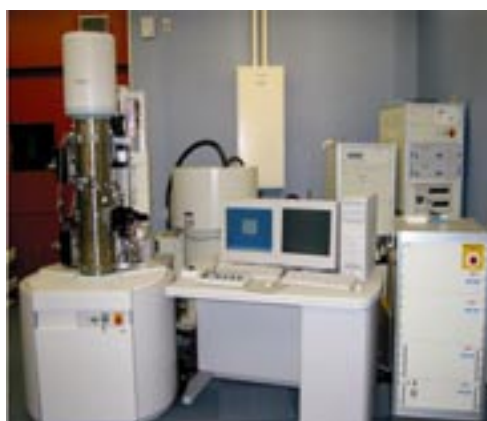
A dedicated scanning transmission electron microscope with atomic sensitivity
