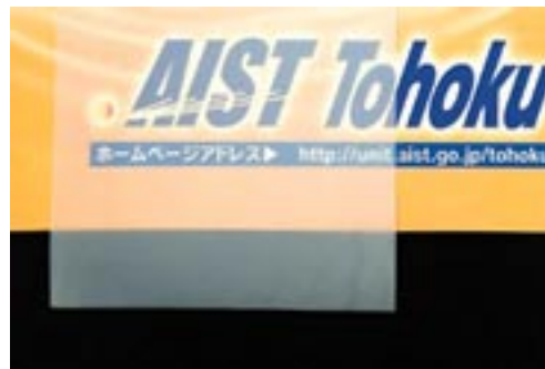
Outlook of the translucent clay film, 0.04mm thick
