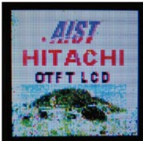
Color liquid crystal display driven by Organic TFT
