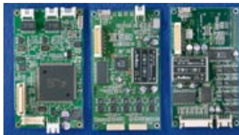
Developed embedded boards(55[mm]×95[mm]) (SH-4 CPU board(left) and stackable peripheral boards)
