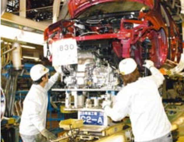
Photo 2 Installing an engine unit
