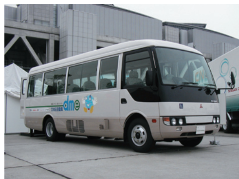
DME powered mini-bus with wheelchair lift
