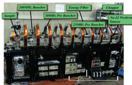
Figure 4. Popular type compact size positron lifetime spectrometer (under development)
