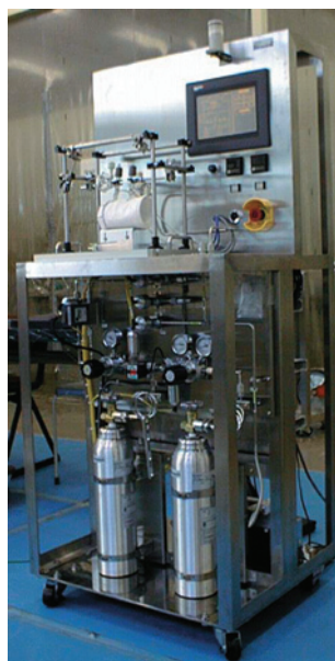
Practical device for the automated manufacture of hyperpolarized xenon gas developed through the AIST research
