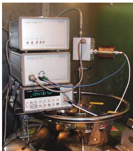
Measurement set-up for a Josephson-based Fast-Reversed DC
