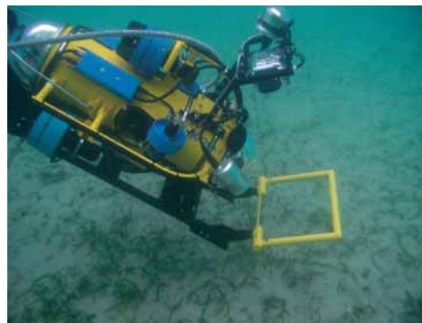
Underwater robot taking the picture of seagrasses within the quadrat frame
