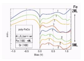
Oscillatory components of the differential conductance of MTJs with ultrathin Fe (100) electrode for various thickness Fe (100) electrodes;Cr(100)(30nm)/ Fe(100)(nML)/AI-O(1.7nm)/FeCo(20nm).
