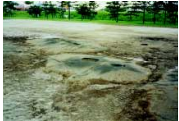
Sand blows on Oshamanbe, Hokkaido, after the 1993 Earthquake off the Southwest Coast of Hokkaido. The maximum diameter of the sand blows is about 2m
