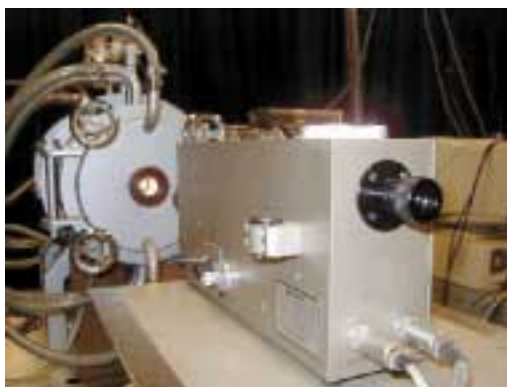
Eutectic point observation by radiation thermometer
