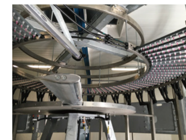
Research on technology to prevent deterioration (erosion) of wind turbine blades caused by raindrops, etc.
