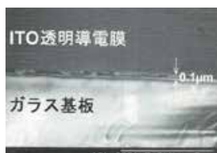
透明導電膜の製造法 Production method for transparent conductive Indium tin oxide (ITO) film
