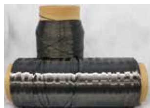
PAN系炭素繊維 Polyacrylonitrile (PAN) based carbon fiber
