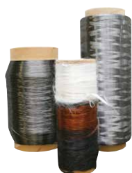
PAN系炭素繊維 Polyacrylonitrile (PAN) based carbone fiber
