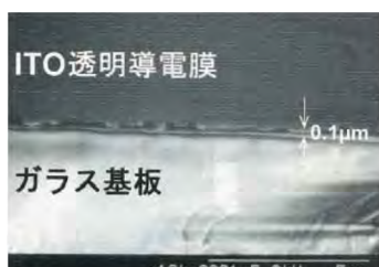
ITO透明導電膜 ガラス基板 透明導電膜の製造法 Production method for transparent conductive Indium tin oxide (ITO) film
