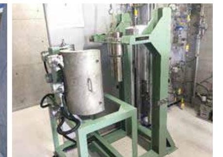
100 MPa Pressure Resistance / 200°C Heat Resistant Reaction Vessel
