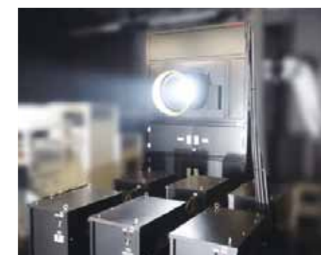
Solar simulator for PV module performance testing and calibration (Solar irradiance emulating and temperature control chamber)
