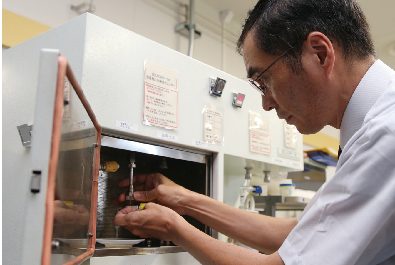
▲ An automated measuring device for testing the moisture-adsorption characteristics of nanoporous ceramics. Without such a device, testing alone would take two to three months.
