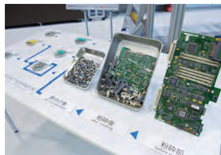
Computer circuit boards classified by types of metal by an automatic separation system
