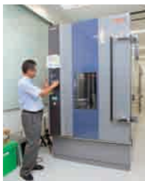
Temperature and humidity test apparatus for developing reliability testing methods.
