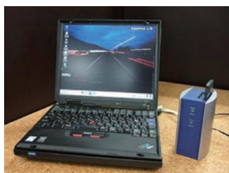
Fig. 6: Router with network-boot function incorporated (right blue box) and KNOPPIX booted through network using it.
