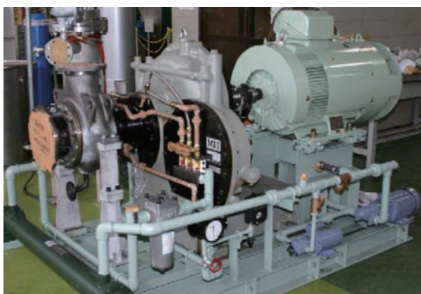
Photo : Small through flow boiler power generation system Courtesy of Kobe Steel, Ltd.
